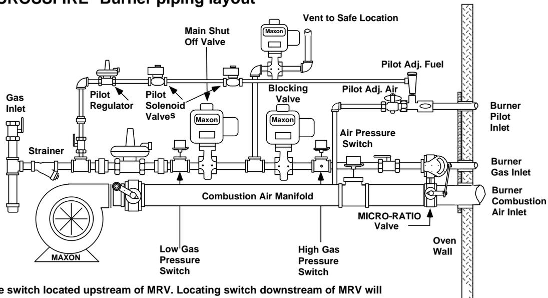
\*Air pressure switch located upstream of MRV. Locating switch downstream of MRV will result in higher air flow than required by the burner at minimum.
