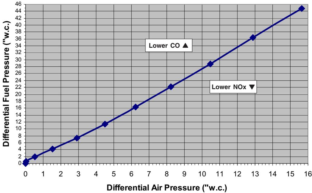
NOTE: Pressure measured at burner test connections; refer to inlet pressure requirements for fan sizing
