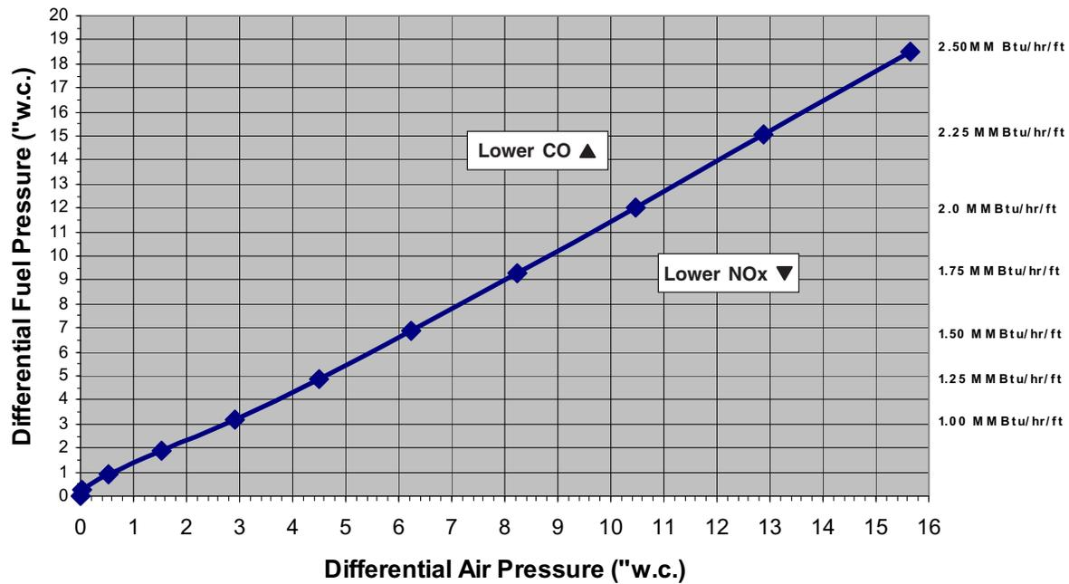
NOTE: Pressure measured at burner test connections; refer to inlet pressure requirements for fan sizing
