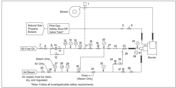
Figure 3.8 - Schematic for #2 Fuel Oil
