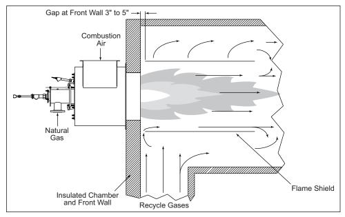
Figure 3.2 - Flame Shield (Typical Example with Gap)
