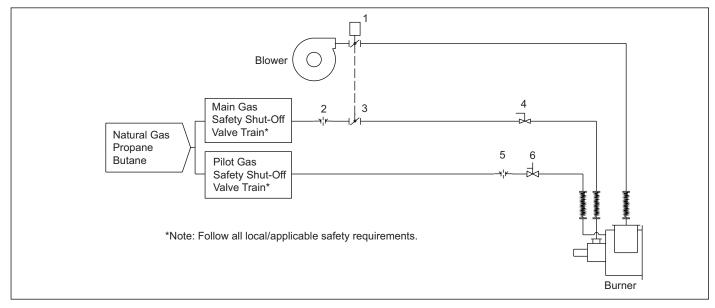
Figure 3.4 - Schematic for Natural Gas, Propane, & Butane
