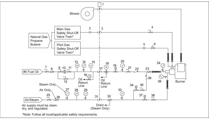
Figure 3.5 - Schematic for Natural Gas, Propane, Butane and #6 Fuel Oil
