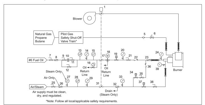
Figure 3.6 - Schematic for Natural Gas, Propane, Butane & #2 Fuel Oil
