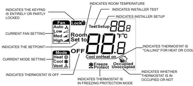
Fan can be selected as manual or automatic 3-speed operation. In Manual mode, the fan is switched to the selected speed via control output Gh, Gm, Gl. While in automatic mode, fan speed depends on the difference between room temperature and setpoint. When room temperature reaches setpoint, valve will be closed and meanwhile, fan will be closed either.
