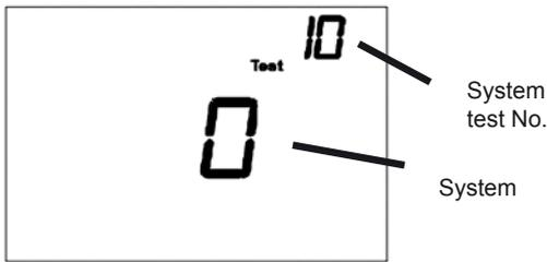
Press and hold ▲ and ▼ buttons 3 seconds to enter test mode.
