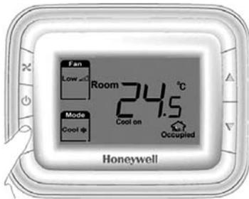
PRESS THE MODE BUTTON TO SELECT HEAT, COOL OR VENT
