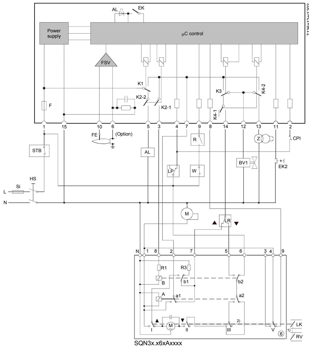
**⚠** If the contacts of switch V welded in position 4 → 9, supervision of the ignition load position would be negated and would not be detected in operation. This means that the circuit is not safety relevant. It is only used for supervision purposes. The user must ensure that, in the event of failure (should the burner ignite at nominal load «NL»), no damage will occur.
