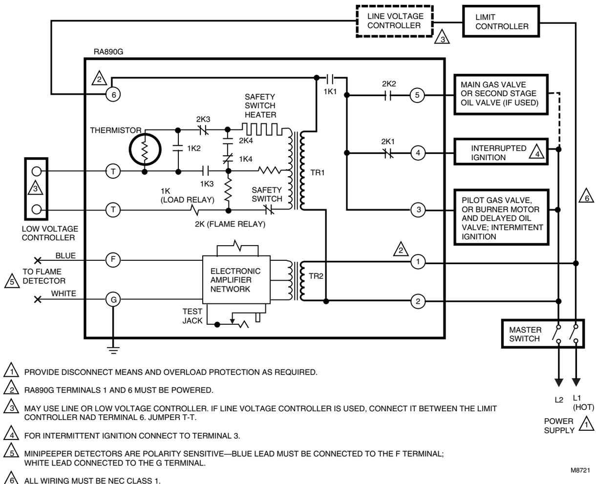
Fig. 6—Flame current check.
